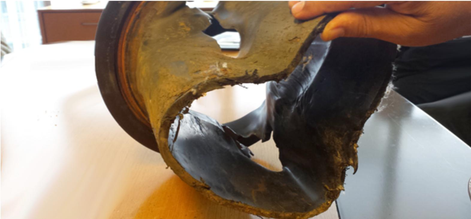
*Collapsed HDPE pull thru liner*
