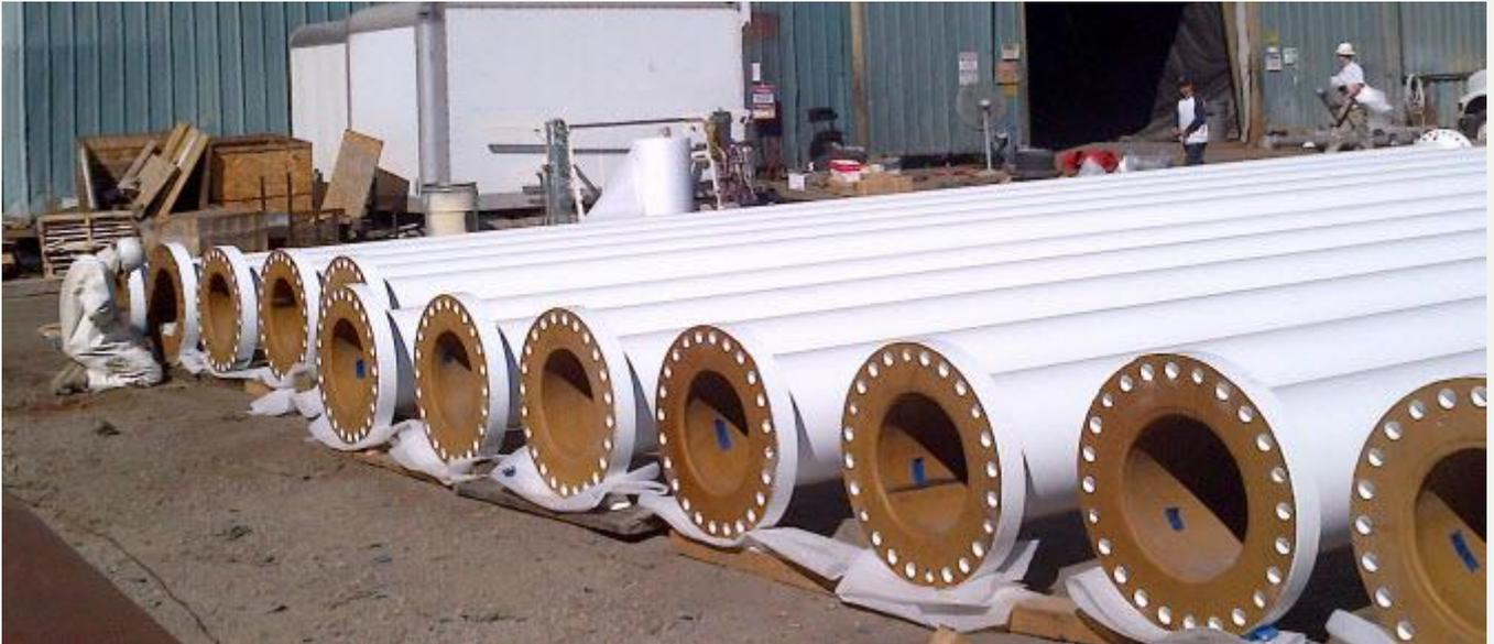
In a growing trend in the mining industry, the mine's process water was derived from the ocean. The corrosive nature of saltwater, the abrasiveness of the slurry, and the high-pressure due to the water being pumped all the way from the sea, made for a very abusive environment. Fluor engineers decided to specify a thick soft rubber lining for the job.
