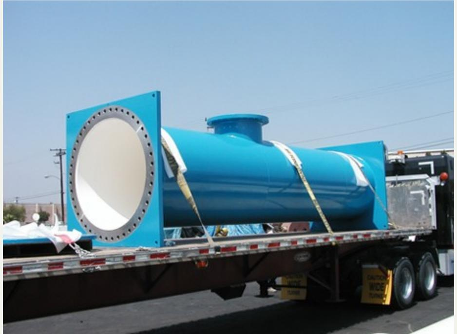
*Vertical pump barrel, ready for delivery to the customer job site*
